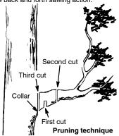
Make the first cut 6 inches (15 cm) from the tree trunk on the bottom of the limb. Use top of guide bar to make this cut. Cut 1/3 through the diameter of the limb.
